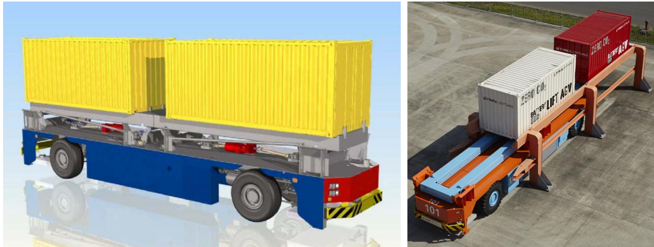
FIGURE 3-6 LIFT AGV WITH TWO TWENTY-FOOT CONTAINERS (LEFT) AND CONTAINERS DEPOSITED ONTO STORAGE RACKS (RIGHT)
